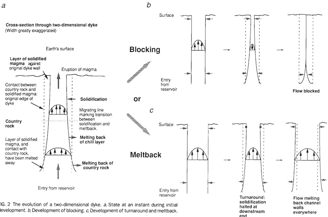
FIG. 2 The evolution of a two-dimensional dyke. *a*, State at an instant during initial development. *b*, Development of blocking. *c*, Development of turnaround and meltback.
