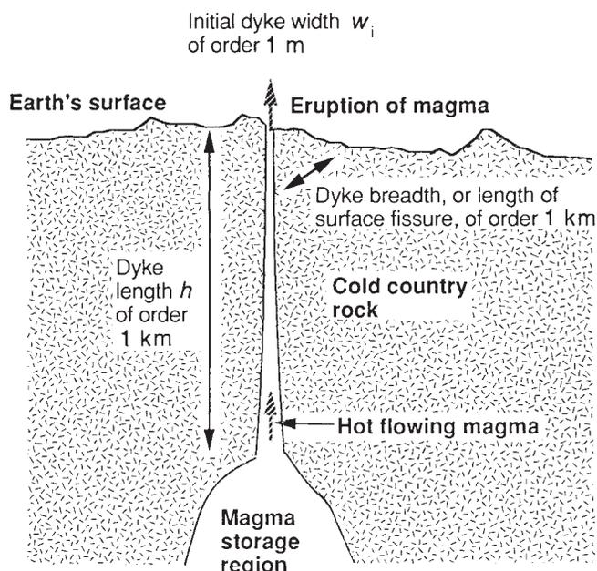
FIG. 1 Cross-section through a typical sheet-like planar dyke. Note that the dyke need not necessarily be vertical.
