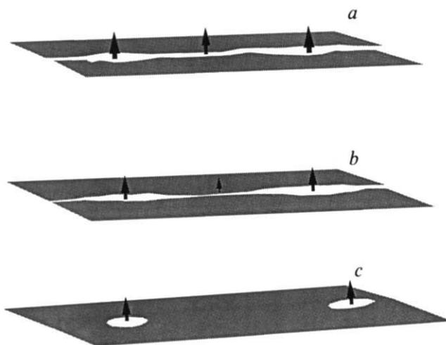
FIG. 4 A schematic (not to scale) diagram of flow localization and development of a surface fissure over time. *a*, initial irregularities of width (which may be small). *b*, faster solidification in narrow regions exaggerates the difference. *c*, flow through isolated vents melts back walls and flow is blocked elsewhere.
