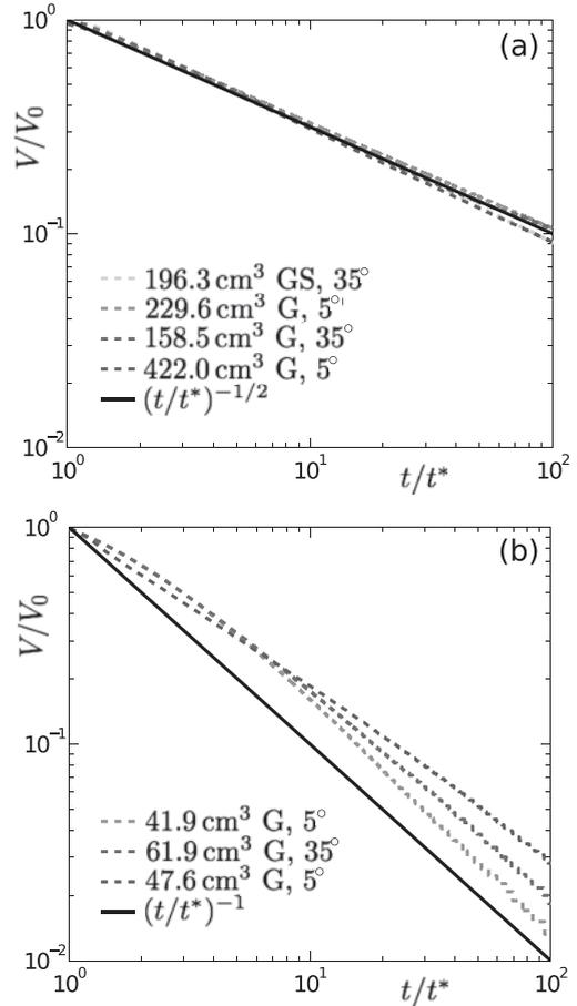
FIG. 3. Proportion of glycerine (G) and golden syrup (GS) remaining along (a) flat edges of a square container and (b) corners of a square container with a wedged base, plotted on logarithmic scales against rescaled time.
