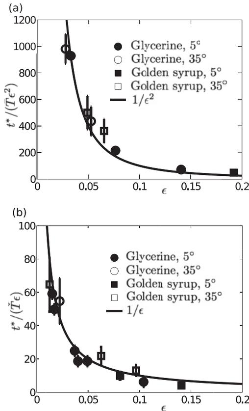
FIG. 2. Rescaled time when fluid begins to pour out of (a) a flat edge of a square container and (b) a corner of a square container with a wedged base, plotted against the proportion of the container initially occupied by the fluid.
