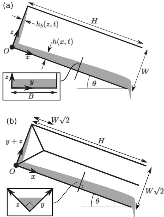
FIG. 1. Sketch of (a) a tipped container of rectangular cross section such that the bulk flow is along two planes and (b) a square container with a wedged base such that the bulk flow is along the wedge and a corner of the container. Each inset shows a cross section of the flow.
