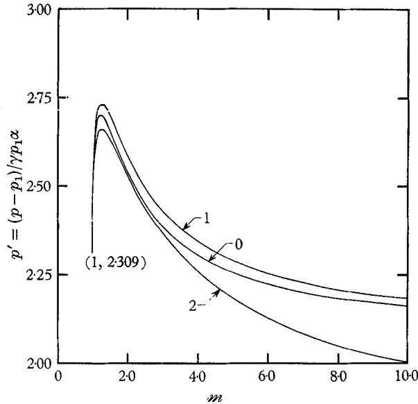
FIGURE 3. The relative pressure on the wedge, just behind the diffracted shock wave, for  $M = 2$  and  $\gamma = 1.4$ . Curves 0 and 1 are based on  $(\delta m/\delta\theta)_0$  and  $(\delta m/\delta\theta)_1$ , respectively; curve 2 is based on the linearized boundary-value problem.  $p_1$  is the undisturbed pressure behind the incident shock wave.
