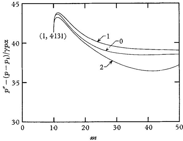
FIGURE 4. The pressure on the wedge, just behind the diffracted shock wave, for  $M = 4$  and  $\gamma = 1.4$ . Curves 0 and 1 are based on  $(\delta m / \delta \theta)_0$  and  $\delta(m / \delta \theta)_1$ , respectively; curve 2 is based on the linearized boundary-value problem.
