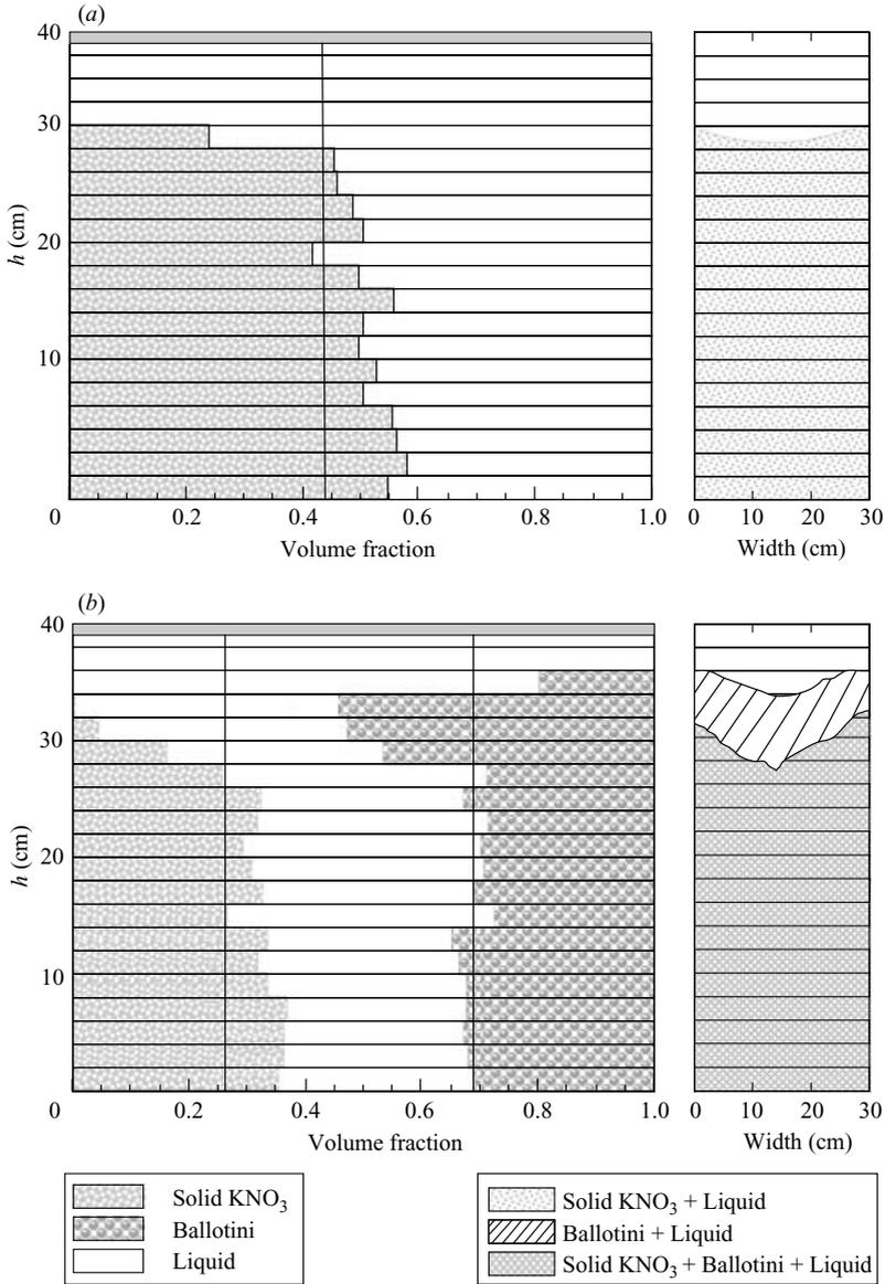
FIGURE 8. The final volume fractions of solid and liquid phases as a function of height, determined from analyses of the residual porous matrices from (a) Expt 2a, initially having a solid matrix composed of pure  $\text{KNO}_3$  with  $\phi_o = 0.437$ , and (b) Expt 3a, initially having a solid matrix composed of a mixture of glass ballotini and  $\text{KNO}_3$ , with  $\phi_g = 0.306$  and  $\phi_s = 0.264$ .
