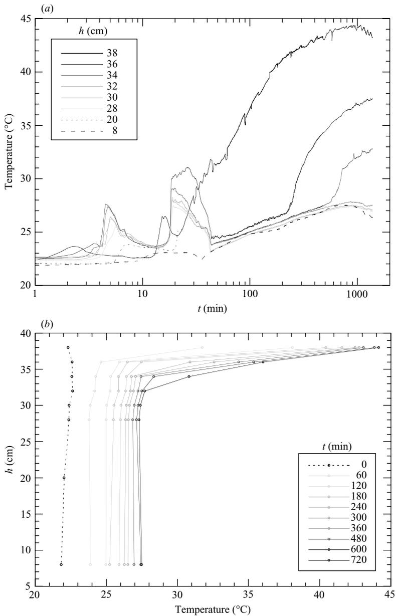
FIGURE 7. The temperature data from an array of eight thermistors at different heights in Expt 2a plotted against (a) time, and (b) height at selected times.
