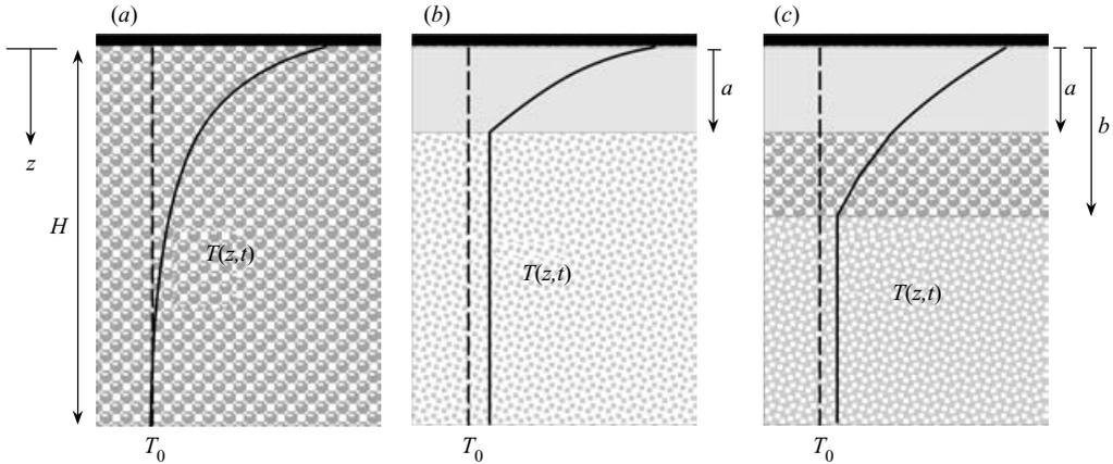
FIGURE 3. Schematic representations of the three experimental variations, including the temperature profile developed in each case. (a) Ballotini in water, (b)  $\text{KNO}_3$  in solution, (c)  $\text{KNO}_3 +$  ballotini in solution.
