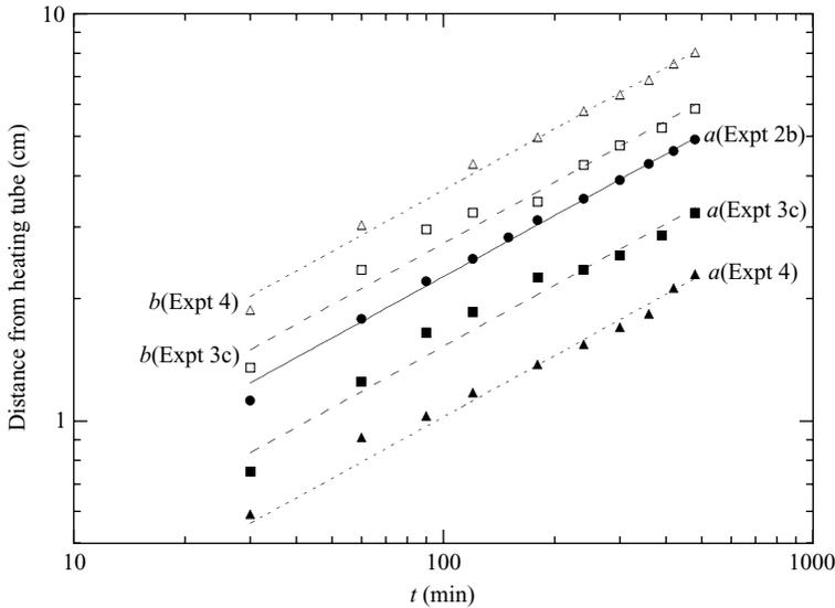
FIGURE 6. The mean height of the interfaces, measured in terms of the distance from the heating tube, plotted as a function of time for experiments with varying initial volume fractions of  $\text{KNO}_3$  as described in table 1. The straight lines through the data points are the individual best-fit curves according to a relationship of  $t^{1/2}$ . Their constants of proportionality are given in table 3.
