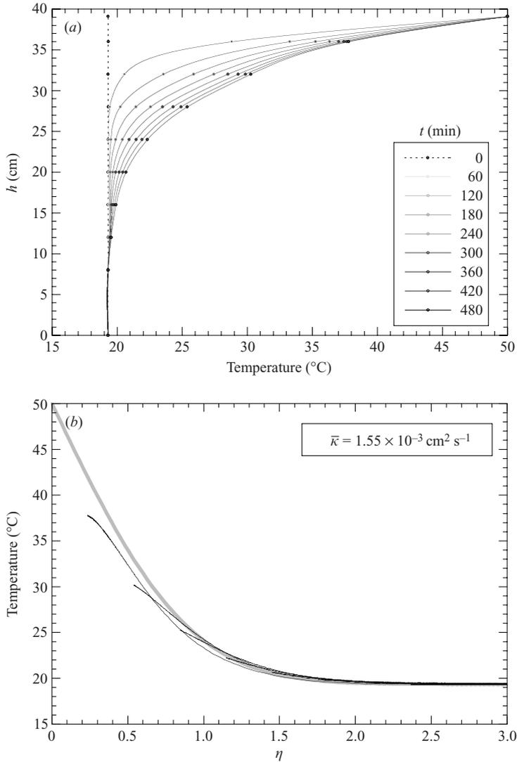
FIGURE 4. (a) Temperature measurements as a function of height at selected times in Expt 1, showing the typical conductive profile developed when a porous bed of glass ballotini immersed in water is heated from above. (b) Temperature as a function of  $\eta$  for the scaled data compared with the theoretical curve given by (2.1).
