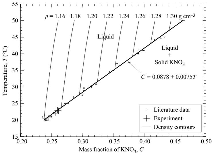
FIGURE 1. Part of the phase diagram for  $\text{KNO}_3$ , with the best-fit linear  $C$ - $T$  relationship to the data, symbolized by  $\circ$ , given by (3.1) for the (super-eutectic) liquidus between  $20^\circ\text{C}$  and  $50^\circ\text{C}$ , including selected density contours in the liquid region (data from Washburn 1962). The initial temperature and concentration of interstitial fluid in the various experiments are indicated by crosses.
