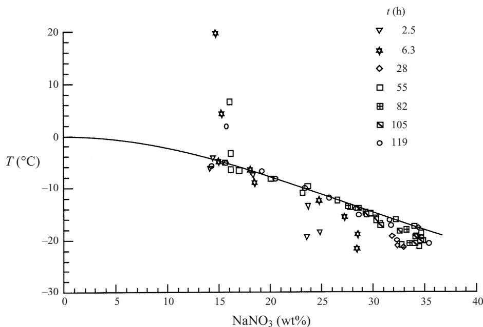
FIGURE 11. Temperature and concentration of  $\text{NaNO}_3$  in the residual liquid for data from experiment 7. The hand-drawn curve is an indication of the section through the liquidus surface along the tie line and then along the cotectic. The discontinuity in slope between these two sections occurs at about 25.5 wt%  $\text{NaNO}_3$ .
