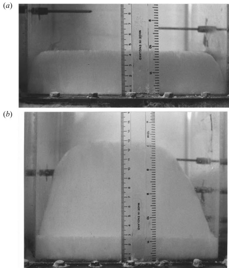
FIGURE 5. Photographs taken from the side during experiment 7. (a) After 5.1 h, the top of the mushy layer is at  $h = 4.7$  cm, while the eutectic front at  $h_E \approx 0.3$  cm is barely visible. (b) After 82.5 h the eutectic front has grown to 2.75 cm and the top of the mushy layer to 14.4 cm. There is a large gap between the mushy layer and the side of the tank at this stage, while the eutectic front extends all the way to the sidewalls.
