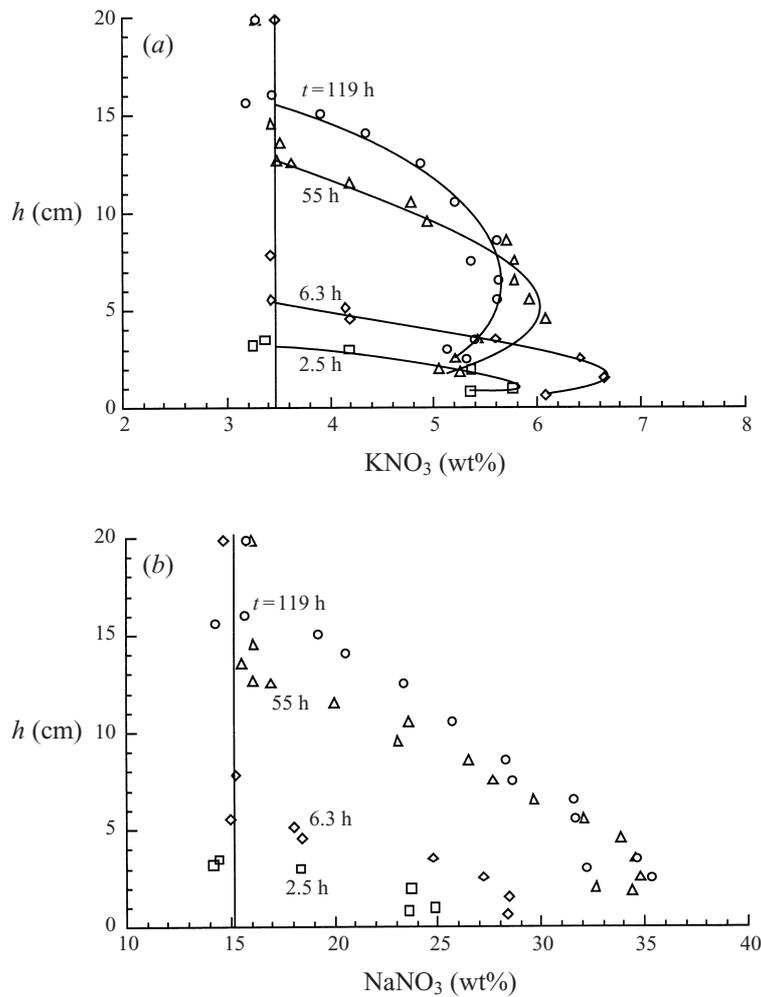
FIGURE 9. The concentrations of (a)  $\text{KNO}_3$  and (b)  $\text{NaNO}_3$  in the residual liquid as functions of height at various times, as indicated. The vertical lines are the initial concentrations.
