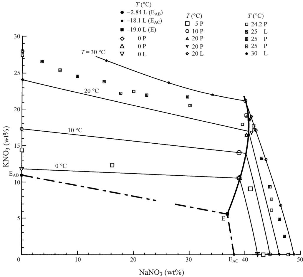
FIGURE 4. The phase diagram for H<sub>2</sub>O-KNO<sub>3</sub>-NaNO<sub>3</sub>. The solubility data, indicated by different symbols, are from Linke (1965) (L) and Protsenko *et al.* (1971) (P). The thick dot-dashed and solid lines are hand-drawn estimates of the cotectic curves based on the available data (shown by the solid or slightly enlarged symbols). Note that the phase diagram is presented using orthogonal coordinates.
