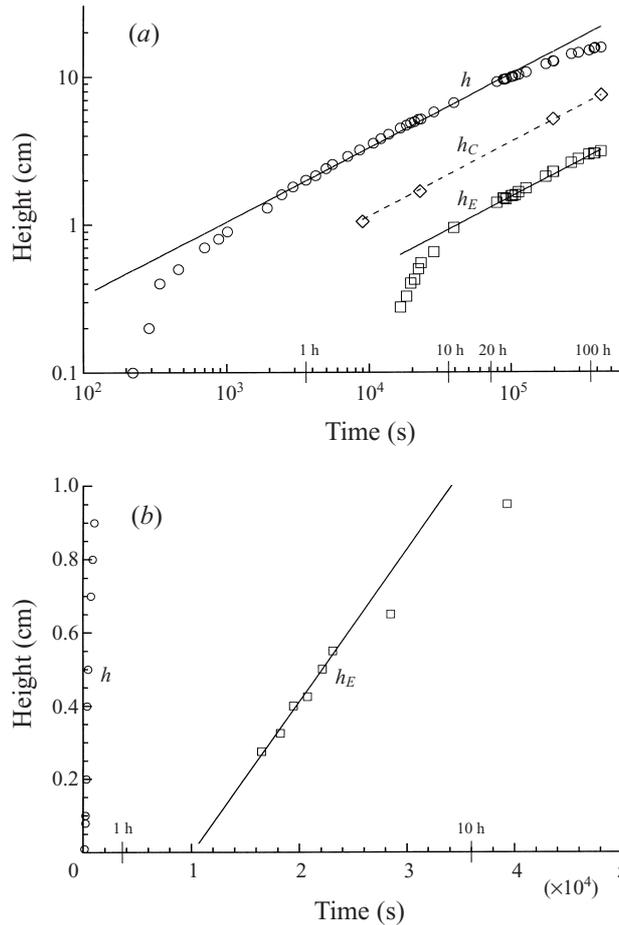
FIGURE 8. (a) The heights of the mushy layer  $h$  and eutectic front  $h_E$  measured directly in experiment 7. The height of the cotectic front  $h_C$  is inferred from the concentration measurements shown in figure 9. The lines are the 'best-fit' lines of slope 0.5 through the appropriate part of the data as discussed in the text and reported in table 1. (b) Close-up of the data on a linear scale to show the delay and the initial linear growth in time at the eutectic front.
