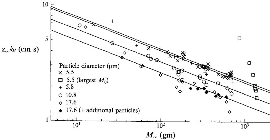
FIGURE 6. Plot of  $z_\infty/\omega$  versus  $M_\infty$  on logarithmic scales for different sized particles and a wide range of stirring frequencies. The best-fit lines to the form  $z_\infty M_\infty^\mu \propto \omega$  have a slope  $\mu$  of  $-0.275$ , and the constant of proportionality is a function of the particle diameter.
