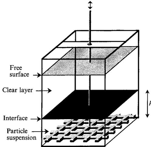
FIGURE 1. Sketch of the stirring box geometry used in the experiments.
