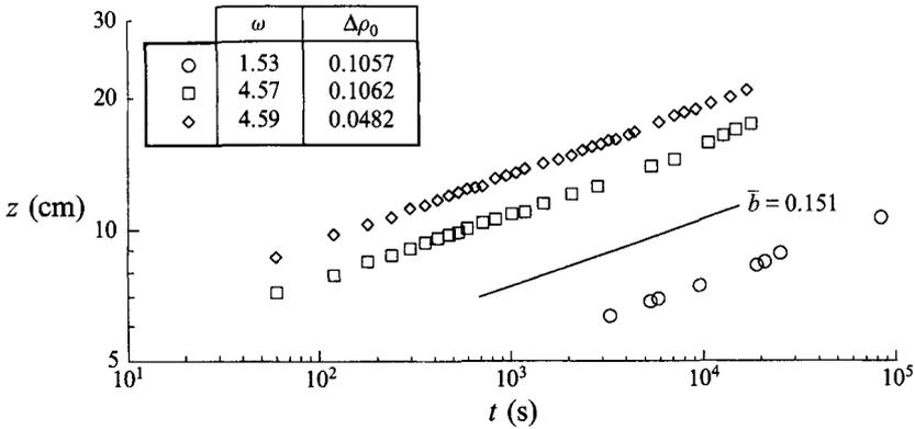
FIGURE 2. The results of three typical experiments with a stirred layer of sugar solution entraining fresh water from above for different values of  $\omega$  and  $\Delta\rho_0$ . The layer depth is plotted as a function of time on logarithmic scales in the form suggested by equation (5) together with a line of slope 0.151. This average slope for all the experiments is included for comparison.
