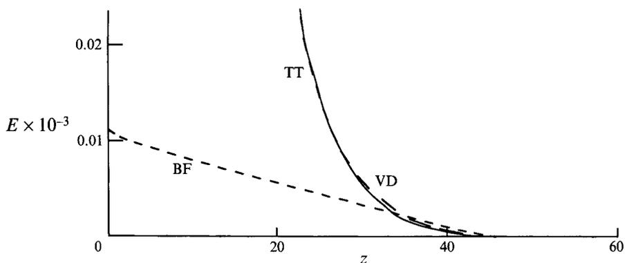
FIGURE 11. Comparison of the turbulent energy transfer (TT), the buoyancy flux (BF) and the viscous dissipation (VD) calculated by Noh & Fernando (1991*a*) as functions of distance from the 'stirring grid' in their numerical computation. Note that the BF dominates the energy balance near the final height, even though it is small there, since it falls off more slowly than VD.
