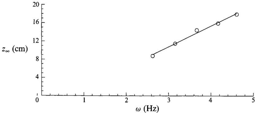
FIGURE 5. The final depth  $z_\infty$  of a sediment layer as a function of stirring frequency  $\omega$  for an individual run in which all the particles of diameter  $5.5 \mu\text{m}$  were held in suspension ( $M_\infty = M_0 = 177 \text{ g}$  and  $\omega > \omega_2$ ).
