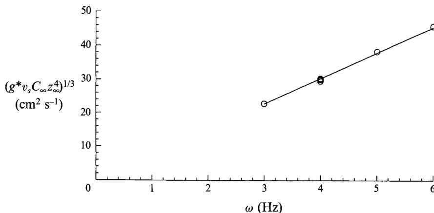
FIGURE 9. The data of E & Hopfinger (1987), scaled according to equation (19). Their experimental results using a different grid size and bottom boundary conditions are well fitted by the same form as our data shown in figure 8, but with a different constant of proportionality.
