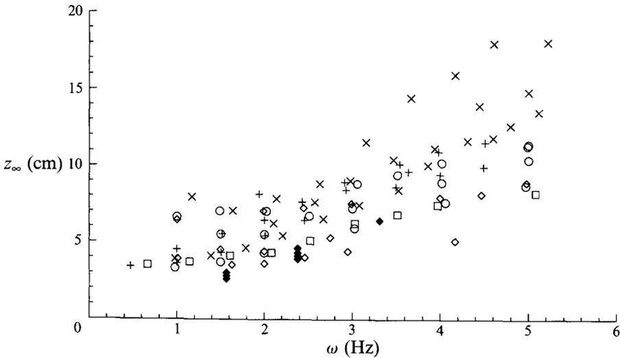
FIGURE 7. Plot of  $z_\infty$  versus  $\omega$  for all the experimental runs with various particle sizes and masses in suspension. Compare this with figure 8, in which the data are scaled in accordance with the theory presented in §4. Symbols as figure 6.
