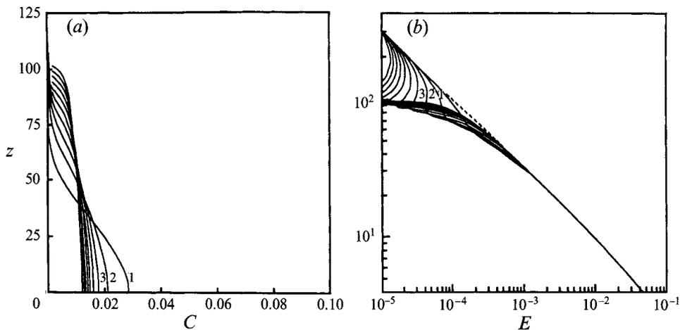
FIGURE 12. (a) The concentration of particles  $C$  and (b) the turbulent energy  $E$  calculated by Noh & Fernando (1991*b*) as functions of time (as marked on the graphs) and distance from the 'stirring grid', for  $G = 10^{-3}$ ,  $R = 10^{-3}$ .
