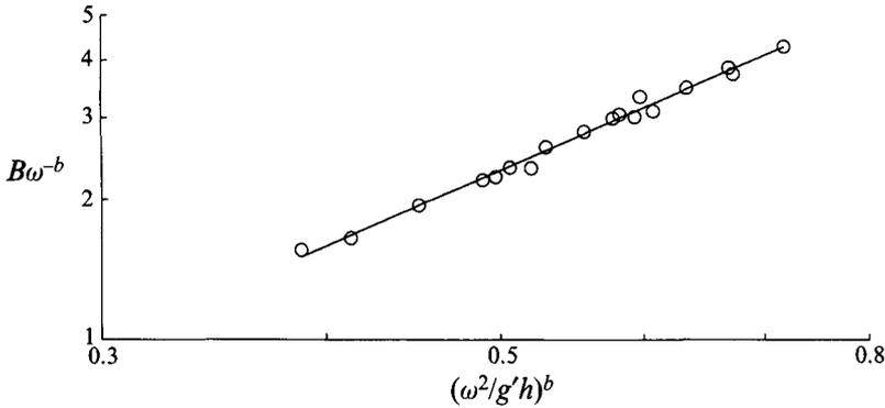
FIGURE 3. Comparison between the experimentally determined values of  $B$  from figure 2 and the corresponding factor in equation (6). Plotting  $B\omega^{-b}$  against  $(\omega^2/g'h)^b$  allows both  $\alpha$  and  $\beta$  to be evaluated using the line of best fit, as described in the text.
